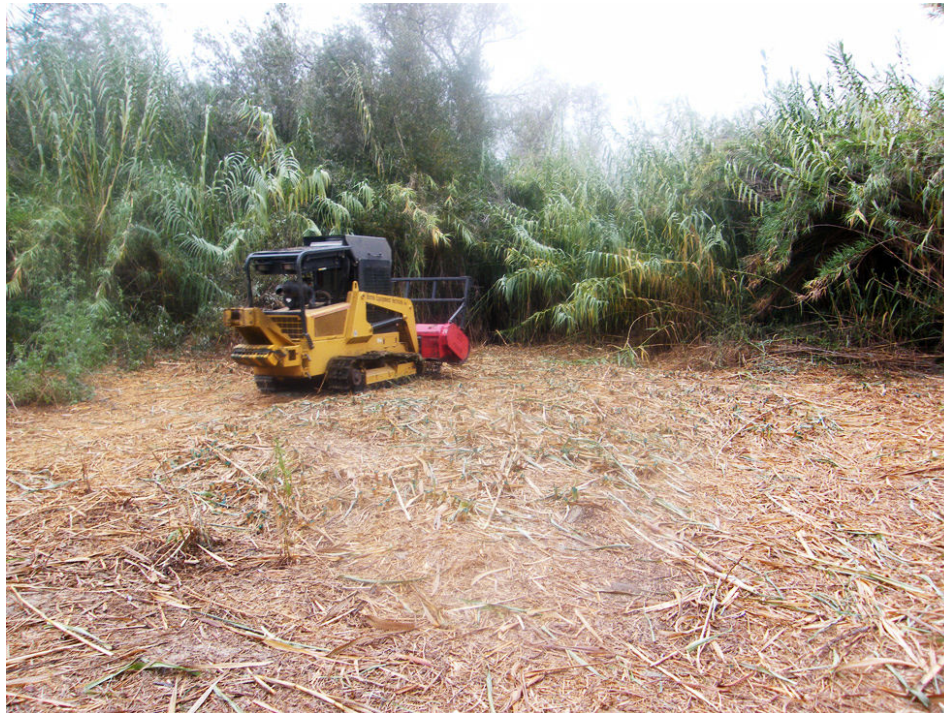
Tractor with forestry masticator used for mowing arundo.
